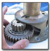
21) Cleaning all bronze center stem. I used wet-dry sandpaper to remove heavy corrosion.
