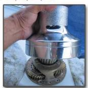
25) Apply Lewmar grease to the bronze stem. 26) Grease and replace washer, bearing, plastic spacer, and second bearing in proper order. 27) Grease gear teeth inside of the drum. 28) Carefully set drum back onto gears. You will feel it engage with the gear sets.
