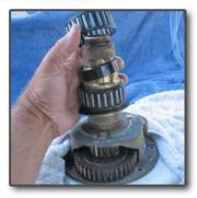
9) Lift off the drum. 10). Inside view of drum. 11) Note corrosion and lack of grease on main shaft.
