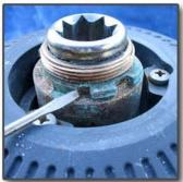
Left to right, 1 & 2): remove screw-on top: To get this moving, I lightly tapped with a hammer against the end of a channel-lock to prevent damage to the cap. 3): Lightly pry off the feeder arm. 4) Lightly tap out retainers – note corrosion from 3 yrs of no maintenance. Watch out that these don't fly over board!
