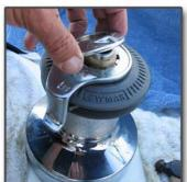
29) Grease center shaft and install. This is as expected, a tightly machined shaft, so not much grease is needed. 30) Insert shaft retainer keys. To get these to seat properly, you may have to raise the center shaft slightly. 31) Install feeder arm in same position as originally set. 32) Screw on cap and hand tighten.
