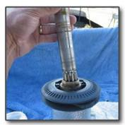
5) I used a little WD-40 to loosen these retainers to get them out. 6) Both retainers, one after wire brushing off the corrosion. 7) Now remove the main center shaft. To get a grip on this, I again used a handle of my channel locks to lift this out since there was no way to grab it. 8). Shaft removed.
