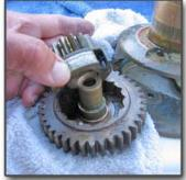
Lt. to rt. 17) First gear assembly - the smaller gear with the pawls just lifts out of the larger gear.
